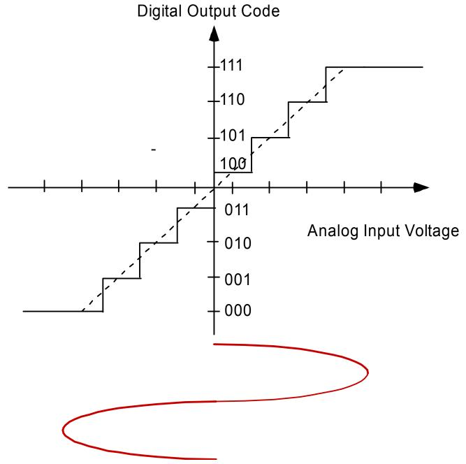
$$SNR_{\text{full scale}} = \frac{(\frac{FS}{2} \frac{1}{\sqrt{2}})^2}{\sigma_q^2} = \frac{(\frac{2^n \Delta}{2} \frac{1}{\sqrt{2}})^2}{\frac{\Delta^2}{12}} = 2^{2n} \frac{12}{8}$$
