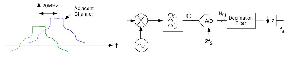
When Adjacent Channel present, most is filtered and suppressed by digital decimation filter *after* ADC.
